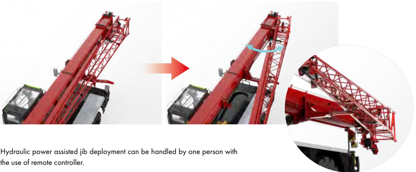
Hydraulic power assisted jib deployment can be handled by one person with the use of remote controller.
